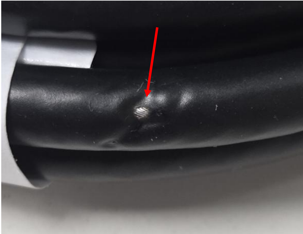
HDMI Cable damaged.
